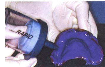
Clip lid on mixing pot and dispense onto fit surface of Replablock
