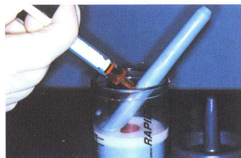
Measure Activator by volume. Trickle down mixing rod
